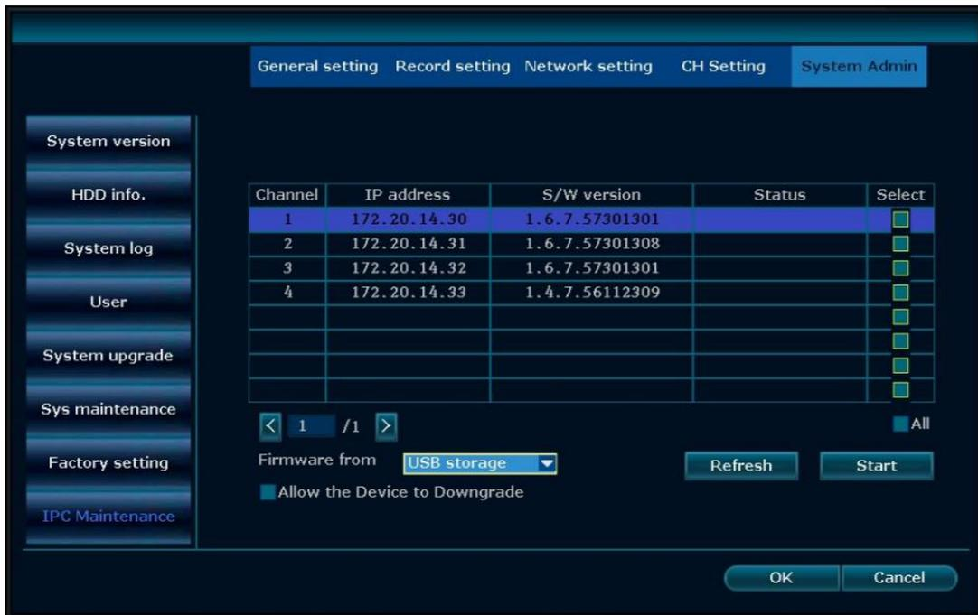
2. Download cameras firmware, copy the .rom firmware file to an USB flash disk's root directory, not in any folder. Plug the USB disk to NVR's USB port.
