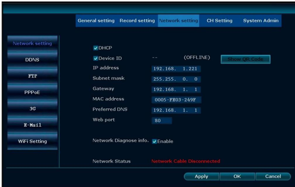
Step2. Enter the NVR's IP address in your IE browser in format http://youripaddress, for example: http://10.0.0.12 (If the default WEB port 80 has been changed e.g. to 100, you'll need to add new port number when input IP address in the browser, for example: <http://10.0.0.12:100>). As shown in below image.
